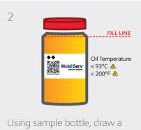
Using sample bottle, draw a representative oil sample from sample point. Secure bottle cap to the sample bottle.
