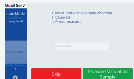
7 First measure the Validation and Day Tank/Fresh cylinder oil sample.
