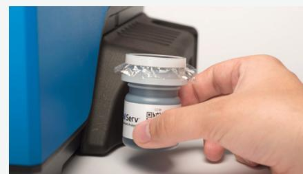
5 Open the sample chamber lid and insert the sample bottle into the sample basket upside down.
